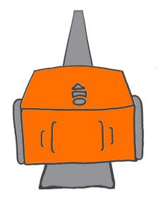
Edison uses a tracking sensor to see the difference between dark and light surfaces. Edison can use this sensor to follow a black line.
