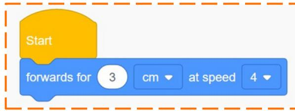
If you ran this program in an Edison robot, would the robot have all the information it needed to know what to do? In other words, does this program tell the robot the direction, distance, distance units and speed to move the motors?
